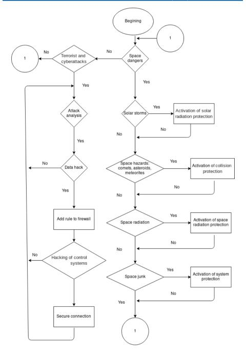
Figure 5: Block diagram for hazards and protection of a Mobile Lunar Base.
