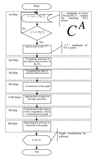
Figure 1: Block diagram of the algorithm for constructing a graph model TA in SN.
