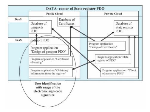
Figure 4: The circuit of model Hybrid Cloud of guiding of State register PDO at level SaaS
