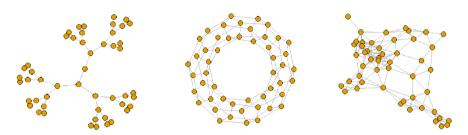
**Figure 1: Three Diagrams of Large-world Networks.**These are highly decentralized systems with dense local connectivity; many steps will be necessary to move information across the system, creating a long average path length.
